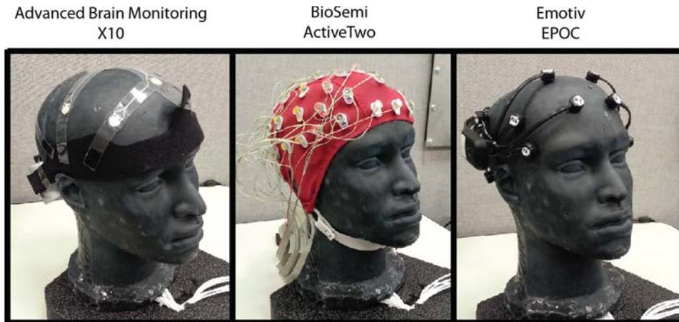
**Figure 2.22 EEG headsets and a phantom head**
